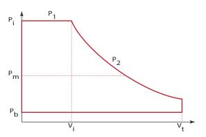
Calculate a rough estimate of the Mean Effective Pressure (MEP) of an ideal expanding steam cycle.
